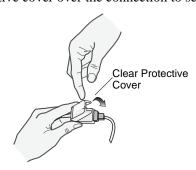
8. Connect the SpO<sub>2</sub> patient cable to the SpO<sub>2</sub> connector on the rear panel of the R Series unit.
