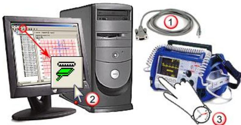
1. Connect the defibrillator to the RescueNet Code Review workstation's serial port. For the M Series/E Series, you must use the ZOLL RS-232 Data Transfer Cable (ZOLL part number 8000-0605-01), which terminates in a female DB9 connector. For the 1600/1700, you must use a ZOLL 1600 Serial Link Cable and Connector (ZOLL part number 8000-1614).
