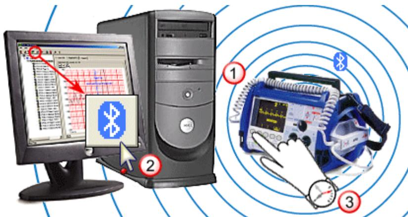
1. Position the defibrillator near the Bluetooth-enabled RescueNet Code Review workstation. Bluetooth is omnidirectional with a range of 20 – 30 feet.
