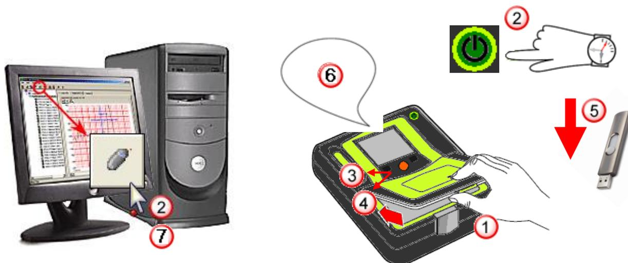
1. Remove the battery cover from the top of AED Pro by releasing the front latch and lifting up on the cover.
