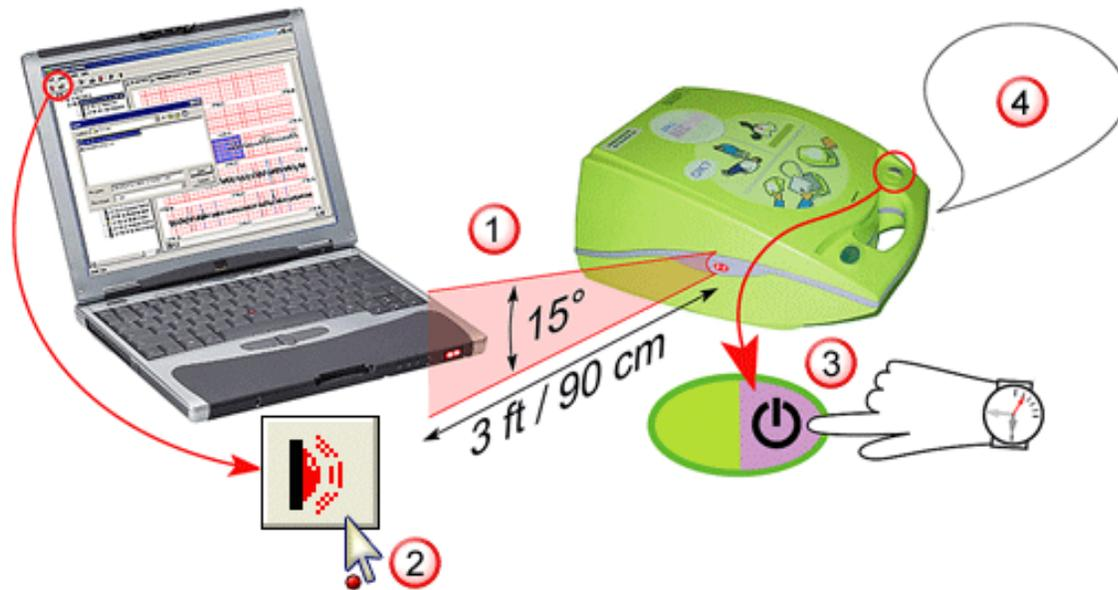
1. Position the AED Plus or AED Pro so that its infrared port lines up with the RescueNet Code Review workstation's infrared port or reader.
