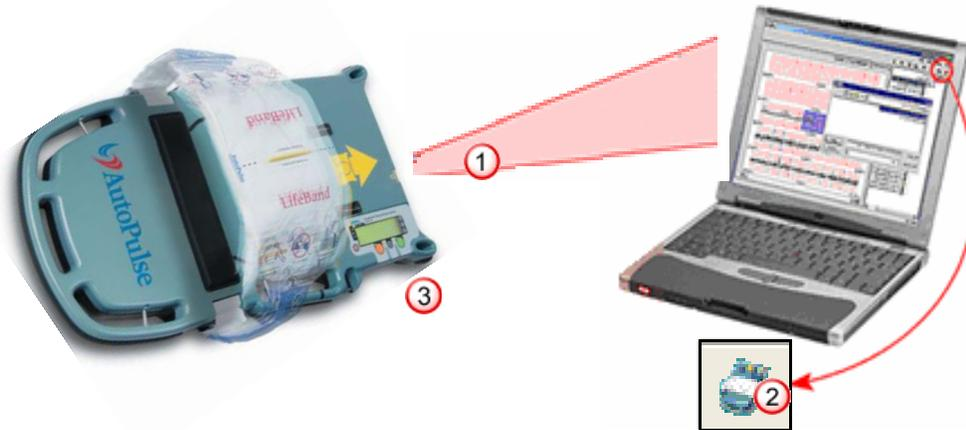
1. Position the AutoPulse so that its infrared port lines up with the RescueNet Code Review workstation's infrared port or reader.
