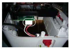
Remove two (2) screws in the areas illustrated to release the capacitor from the unit.
