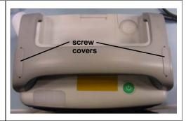
Remove four (4) screws (2 on each handle) and remove the handle.
