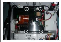
Remove red and white multi-function cable connector from the ECG board in the area illustrated.
