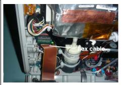
**8** Disconnect the three power cable connectors (battery (black), AUX (white), and defibrillator (red)).
