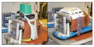
Figure 2 – The piston-driven (left) and load-distributing band (right) systems shown applied to the calibrated mannequin.
