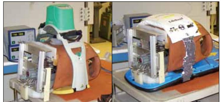
Figure 2 – The piston-driven (left) and load-distributing band (right) systems shown applied to the calibrated mannequin.
