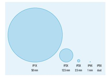
To get some notion of how big the "foreign objects" being described in each of these ratings really are, the diagram above illustrates actual particle sizes. It shows that an AED like the Philips HeartStart OnSite, because it has a rating of IP21, is in danger of being compromised by a small pebble about 12.5 millimeters (mm) in diameter.
