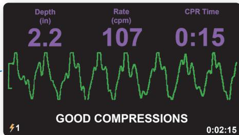
The ZOLL AED 3 BLS can be easily configured to show the CPR Dashboard™ only, or both the CPR Dashboard and ECG. Depth and rate indicators are highlighted in red if the compression rate is too slow and/or the depth is too shallow when in adult rescue mode.
