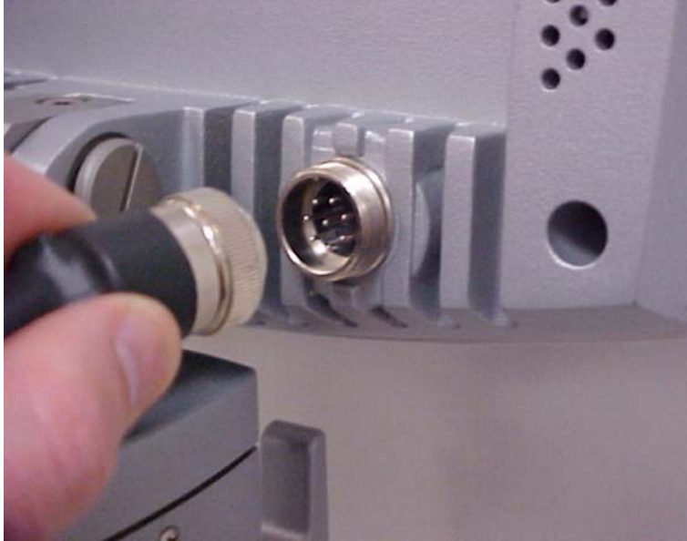
Figure 4.76. The Hirose Connector – Rear of the Display Head
