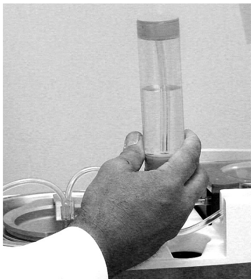
Figure 4.44. Hold the Air Trap Upside Down
