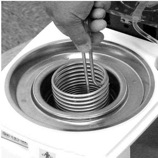
Figure 4.37. Installing the Heat Exchange Coil
