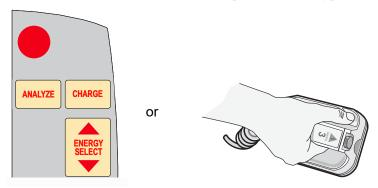
To abort charging and increase or decrease the selected energy after the CHARGE button has been pressed, use the ENERGY SELECT buttons on either the defibrillator front panel or the sternum paddle. Press the CHARGE button again to charge the unit.
