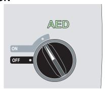
The unit beeps 4 times to indicate that it has passed the power on self test, and the green AED label and the ON mode selector light up on the front panel.
