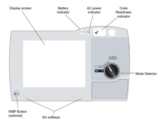
Figure 2-1. R Series Front Panel (AED Mode)
