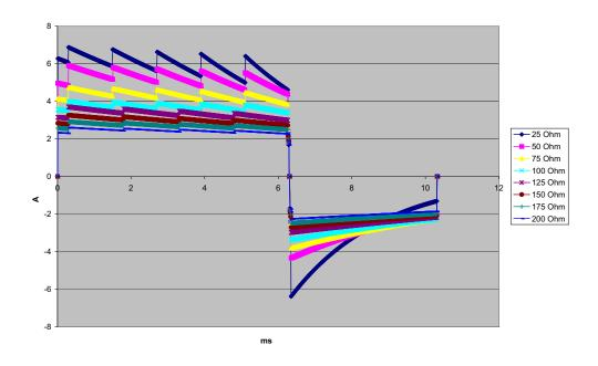
Figure A-12. Rectilinear Biphasic Waveform at 10 Joules
