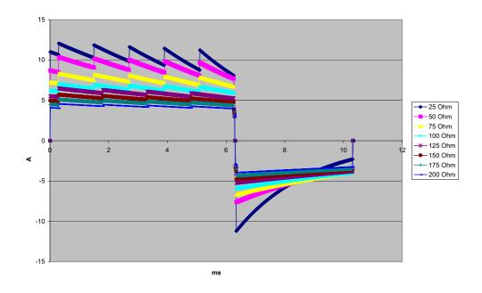
Figure A-9. Rectilinear Biphasic Waveform at 30 Joules
