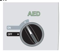
The unit beeps 4 times to indicate that it has passed the power on self test, and the green AED label and the ON mode selector light up on the front panel.
