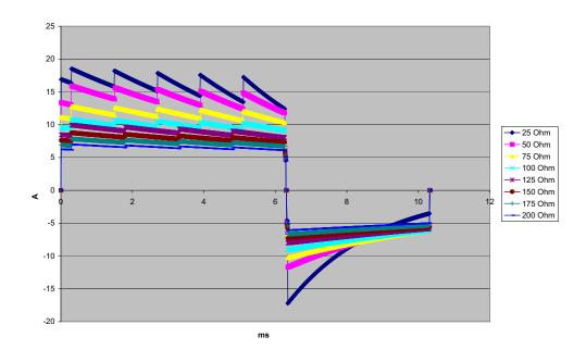
Figure A-7. Rectilinear Biphasic Waveform at 70 Joules
