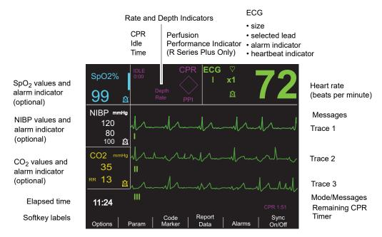
Figure 2-3. R Series Display Screen (shown in manual mode with optional  $SpO_2$ , NIBP and  $CO_2$  monitoring)
