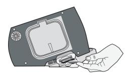
Figure 12-1. Inserting Compact Flash Card
