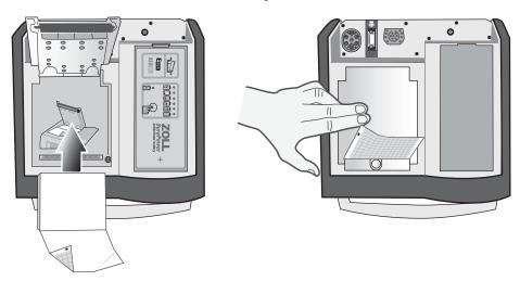
Figure 13-6. Inserting the Paper and Closing Printer Door
