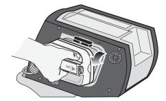
Figure 2-7. Releasing the Paddles
