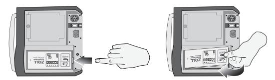
Figure 2-13. Removing a Battery Pack
