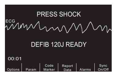
A continuous tone sounds for 50 seconds, followed by an intermittent beeping for 10 seconds. You must deliver the shock within this 60 second interval, or the defibrillator will disarm itself.
