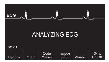
An *ANALYZING ECG* message is displayed for 6 to 12 seconds while the patient's ECG is analyzed. Once the analysis is completed, the unit indicates whether or not a shock is advised.
