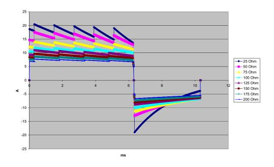
Figure A-5. Rectilinear Biphasic Waveform at 85 Joules
