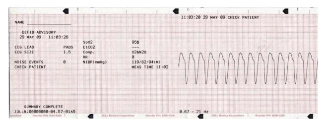
Figure 11-7. VF Alarm Activated Format
