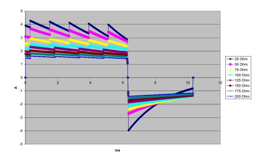
Figure A-18. Rectilinear Biphasic Waveform at 4 Joules
