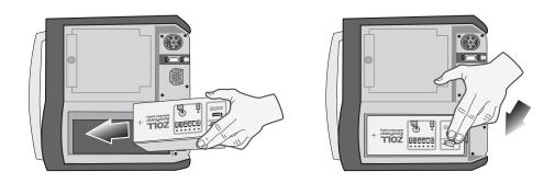
Figure 2-14. Installing a Battery Pack
