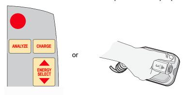
To abort charging and increase or decrease the selected energy after the CHARGE button has been pressed, use the ENERGY SELECT buttons on either the defibrillator front panel or the
