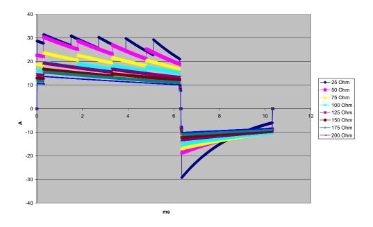
Figure A-1. Rectilinear Biphasic Waveform at 200 Joules
