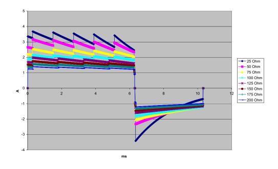
Figure A-19. Rectilinear Biphasic Waveform at 3 Joules
