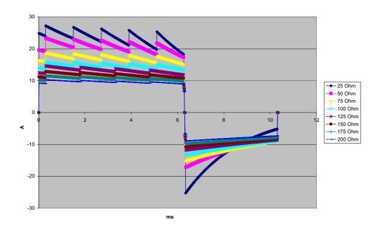
Figure A-2. Rectilinear Biphasic Waveform at 150 Joules
