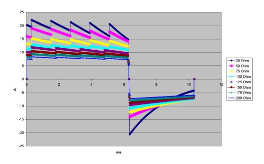
Figure A-4. Rectilinear Biphasic Waveform at 100 Joules
