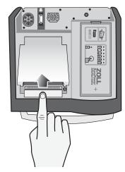
Figure 13-5. Opening the Printer Door
