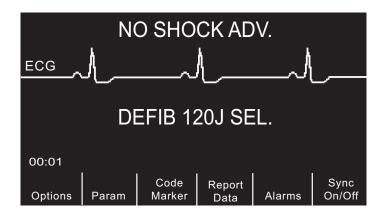
When a nonshockable rhythm is detected, the unit displays a *NO SHOCK ADV*. message. Follow the local protocols to continue CPR or other life support, and re-analyze the ECG at appropriate intervals.
