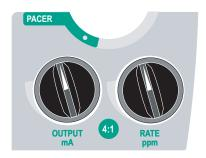
**Note:** When the unit is switched out of PACER mode into Manual mode and then switched back to PACER mode, within 10 minutes the pacer settings remain unchanged.
