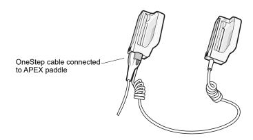
Figure 2-9. OneStep Cable Connected to APEX Paddle
