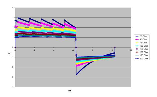
Figure A-20. Rectilinear Biphasic Waveform at 2 Joules
