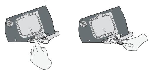
Figure 12-2. Removing a Compact Flash Card
