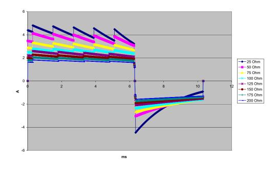
Figure A-17. Rectilinear Biphasic Waveform at 5 Joules
