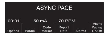
Pace stimuli are also delivered asynchronously whenever there is an *ECG LEAD OFF* condition. Due to the lead off condition, no ECG waveforms will be displayed when pacing by this method. Use other means to determine capture such as checking the patient's pulse.
