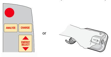
If both **SHOCK** buttons on the paddles are depressed when the **CHARGE** button is activated, the unit does not charge and a *RELEASE SHOCK BUTTON* message appears on the display.
