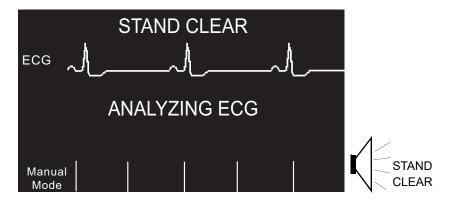
An ANALYZING ECG message is displayed while the patient's ECG is analyzed. Once the analysis is completed, the unit indicates whether or not a shock is advised.
