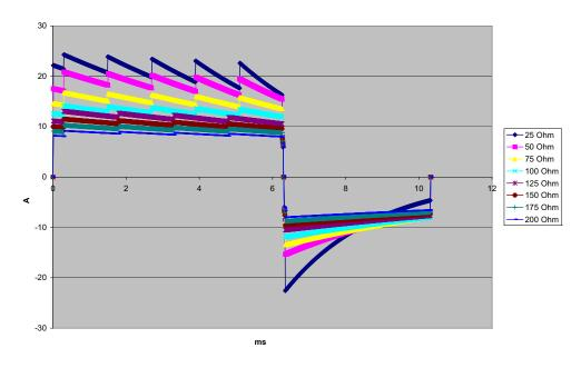
Figure A-3. Rectilinear Biphasic Waveform at 120 Joules
