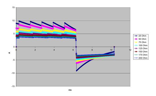
Figure A-10. Rectilinear Biphasic Waveform at 20 Joules
