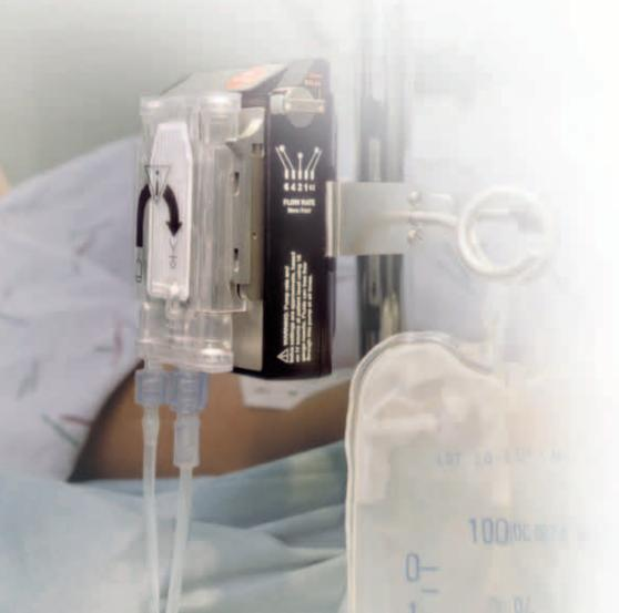
The unique pump mechanism, one-way valves, and air-eliminating membranes built into the cartridge allow the Power Infuser to operate in any orientation.
