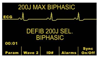
Upon power-up **M Series** units equipped with the Rectilinear Biphasic Waveform Defibrillator Option automatically default to the 120 Joule setting. In units with automatic progressive energy selection enabled, Shock No. 1 is set at 120J; Shock No. 2 is set at 150J and Shock No. 3 is set at 200J. These are the default energy settings. They may be modified following the instructions in the **M Series** Configuration Guide.
