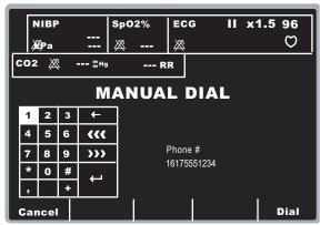
Note: If at least one digit has been entered, pressing the Dial softkey or highlighting the Enter (→) key on the keypad and pressing the Commit (⊙) key dials the entered phone number and displays the following screen:
