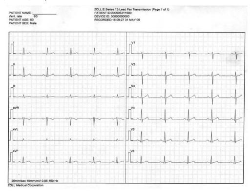
**Note:** This format is not available transmitted via FAX from a Bluetooth device and the ZOLL Data Relay server. **Direct FAX** must be selected in the System Configuration menu (see page 17) in order to be able to send in this format.
