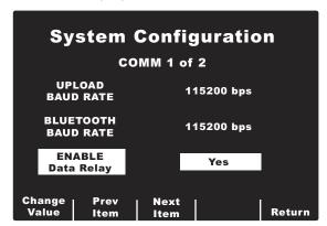
Using the Prev Item and Next Item softkeys on the screen, scroll to Bluetooth Net Server List and press the Change Value softkey. The unit displays a list of current servers.
