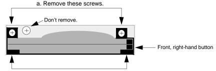
b. Grasp these tabs and pull modem bracket up and out.
