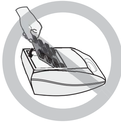
Figure 10: DO NOT install battery assembly this way.
