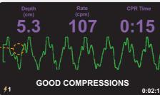
The AED 3 BLS can be easily configured to show the CPR Dashboard<sup>™</sup> only, or both the CPR Dashboard and ECG. Depth and Rate indicators are highlighted in red if the compression rate is too slow and/or the depth is too shallow when in adult rescue mode.
