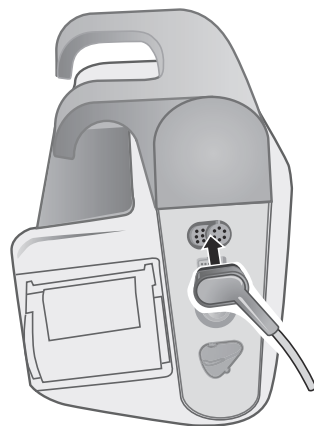
Figure 14-2 Connecting the 12-Lead ECG Cable
