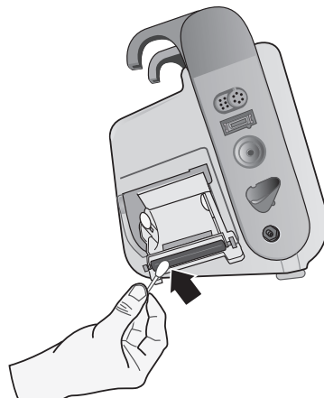
Figure 26-3. Cleaning the Print Head
