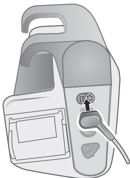
Figure 6-3 Connecting ECG Cable to X Series Advanced Unit
