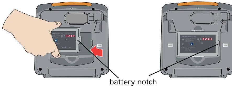
The AED issues a *BATTERY REPLACED* prompt and automatically initiates a self test.
