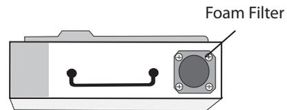
1. Carefully remove the Foam Filter using a hemostat or tweezers.
