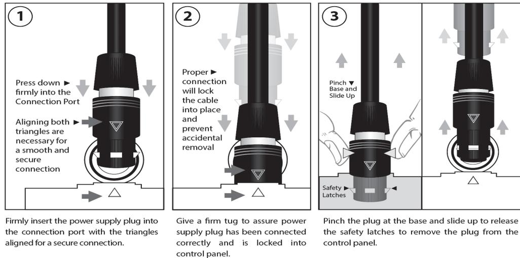
**Figure 3-4 Connecting and Disconnecting the Power Supply**
