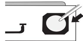
5. **Insert the lower segment of the Compressor Inlet Fitting Assembly into the device, making sure that its alignment pin mates.**
