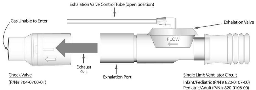
**Figure 6-2 Check Valve Connection To Patient Circuit**
