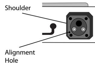
6. **Set the upper segment of the Compressor Inlet Fitting Assembly into the lower segment, making sure that its alignment pin mates.**
