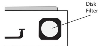
4. Remove the Disk Filter using the hemostat or tweezers and replace it with a new, clean filter. Make sure that the filter sits flat on the shoulder in its recessed area.
