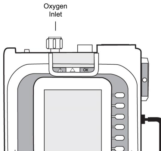
**Figure 3-2 Oxygen Inlet**
