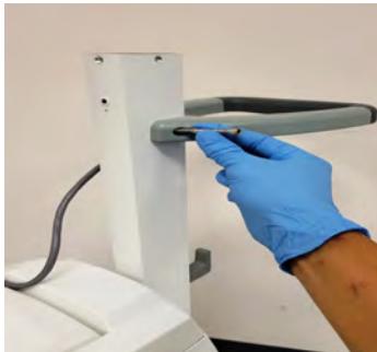
Figure 3.2. Use the long bolt and center screw to attach the handle
