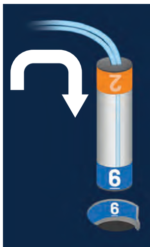
Figure 4.48. Insert air trap into air trap chamber
