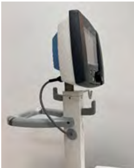
Figure 3.4. Console with front and rear accessory hooks attached
