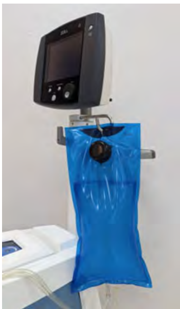
Figure 4.41. Pre-attached reservoir bag on hook for surface pad use
