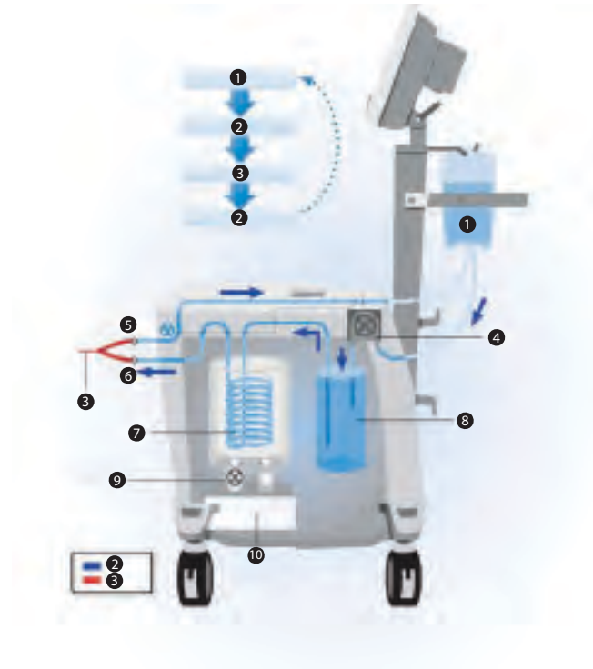
Figure 2.1. Simplified Flow Diagram: Saline Flows in a Closed-Loop Circuit
