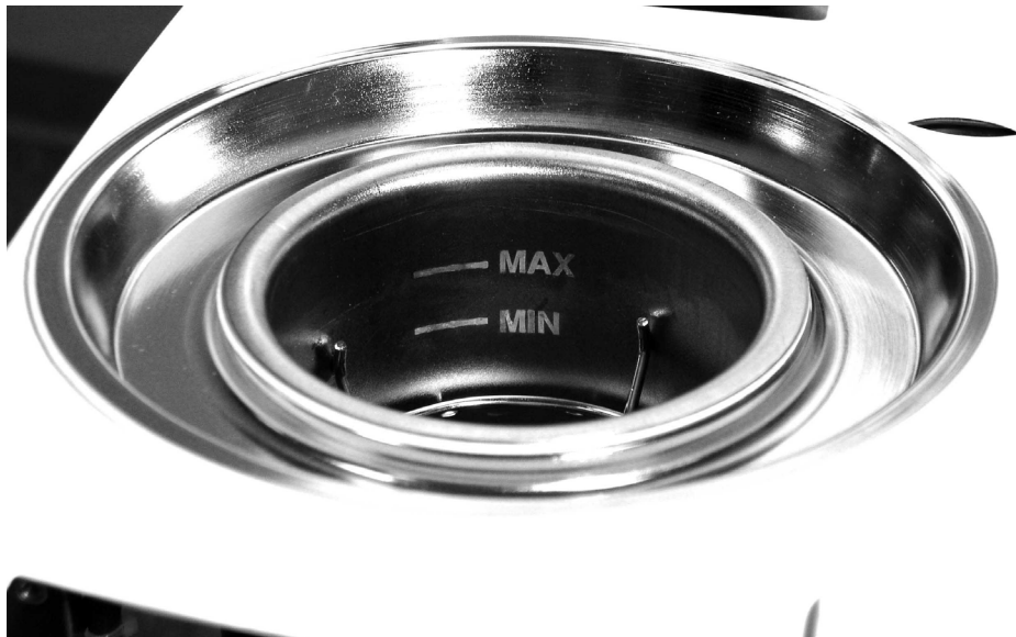
Figure 4.35. Coolant Well Liquid Level Indicator Lines
