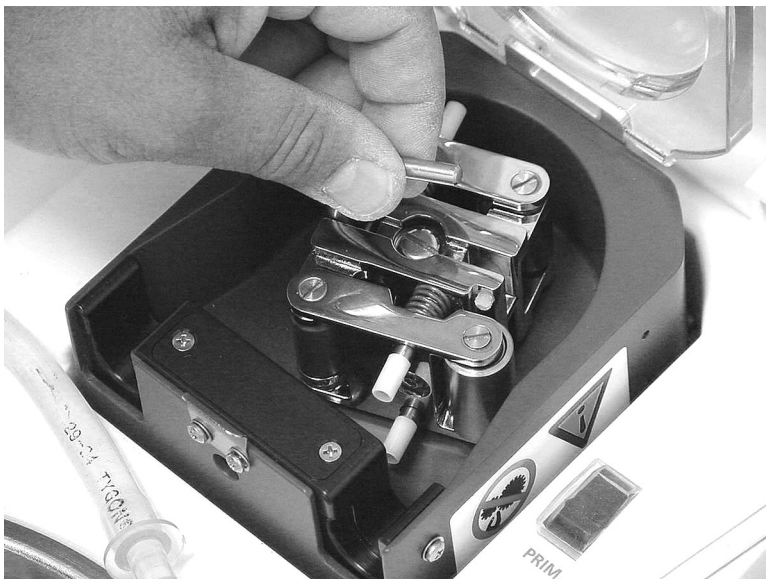
Figure 4.39. Lift the Pump Rollers Handle
