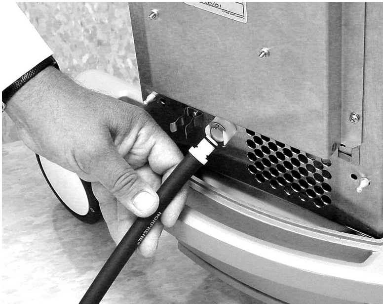
Figure 7.3. Push Hose Into Drain Coupler
