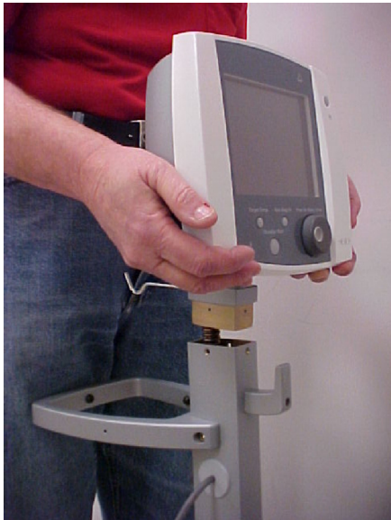
Figure 3.4. Attach the Display Head to the Mast
