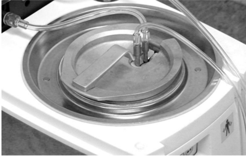
Figure 4.42. Replace the Cap on the Coolant Well
