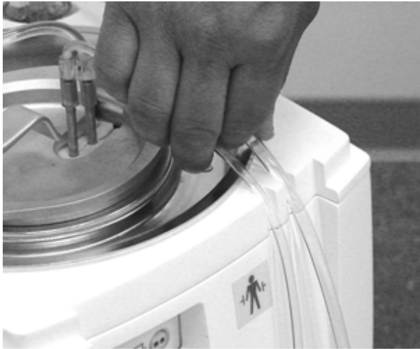
Figure 4.46. Route the Tubing Out of the Console
