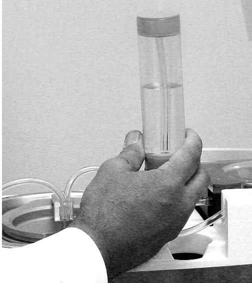
Figure 4.44. Hold the Air Trap Upside Down
