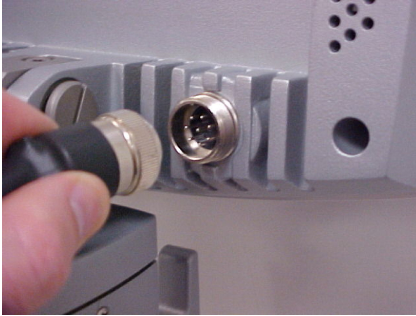
Figure 3.5. Plug the Control Cable Into the Socket
