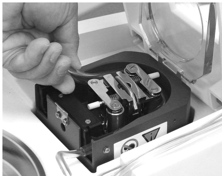
Figure 4.41. Pump Tubing Installation
