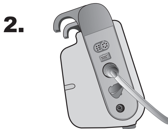
Attaching a Dual Lumen Hose to the Propaq M Unit
