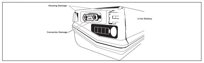
Figure 5-1 Examples of a damaged Battery connector and housing
