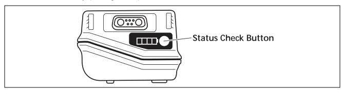
Figure 4-1 AutoPulse Li-Ion Battery Status Check Button and Status LEDs
