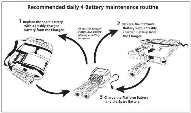
Figure 4-3 Four Battery rotation
