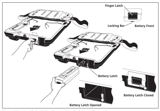
Figure 4-2 AutoPulse Li-Ion Battery Installation and Removal
