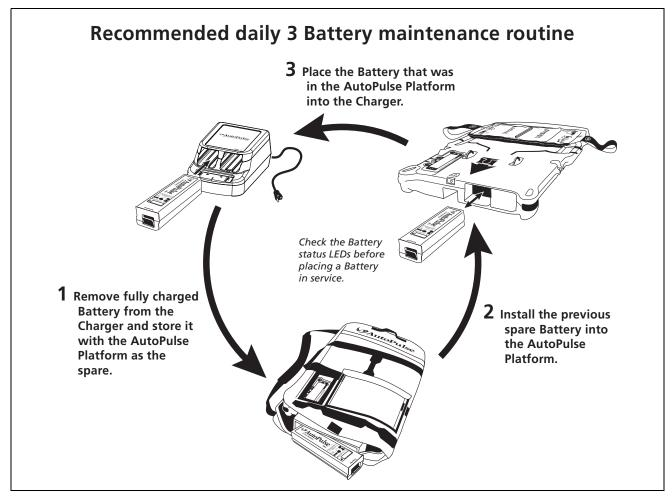
Figure 4-4 Three Battery rotation
