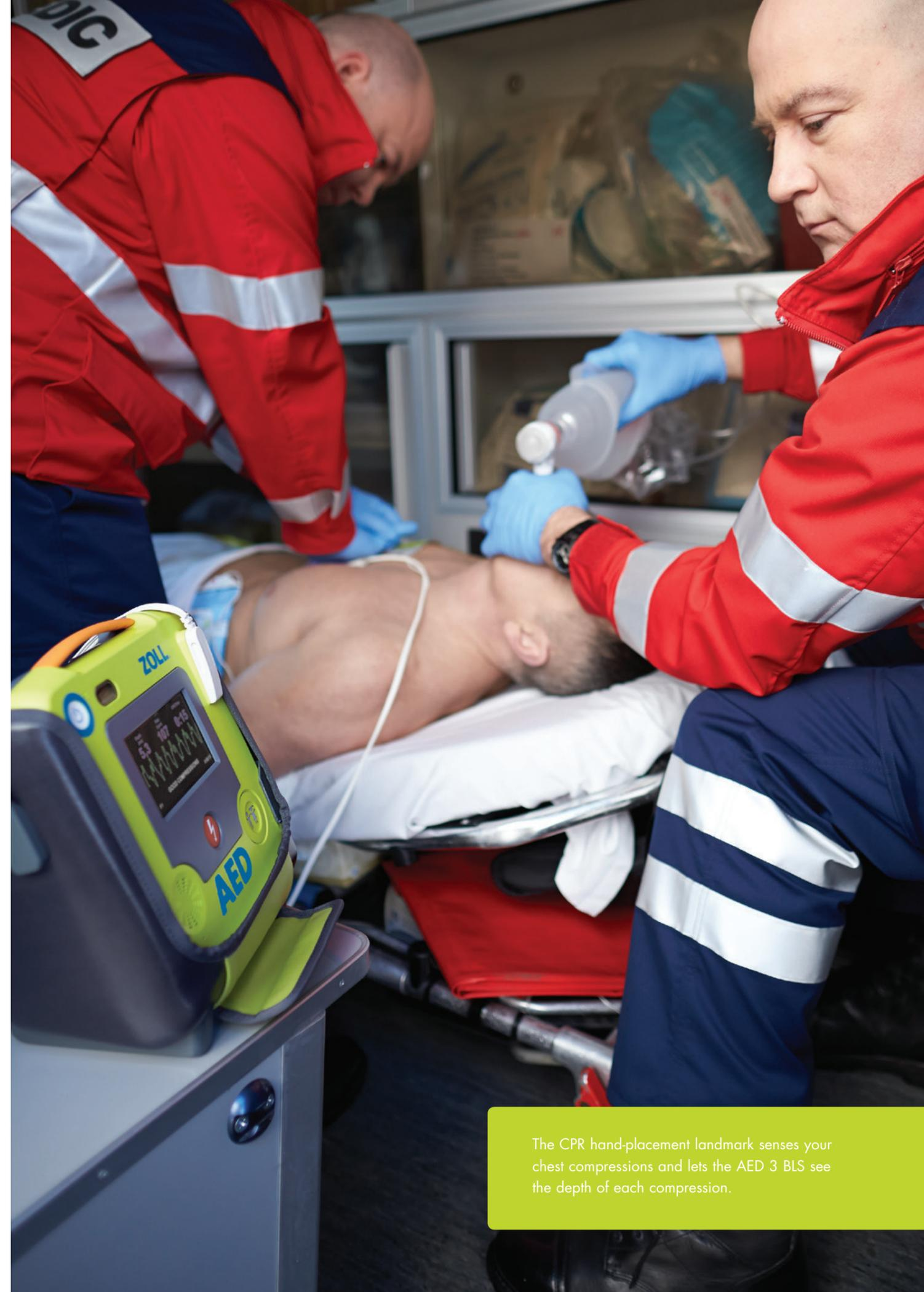
The CPR hand-placement landmark senses your chest compressions and lets the AED 3 BLS see the depth of each compression.
