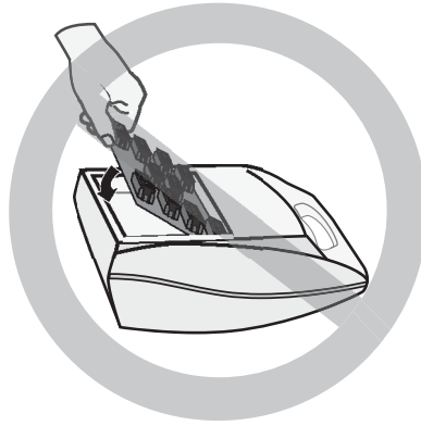
Figure 10: DO NOT install battery assembly this way.
