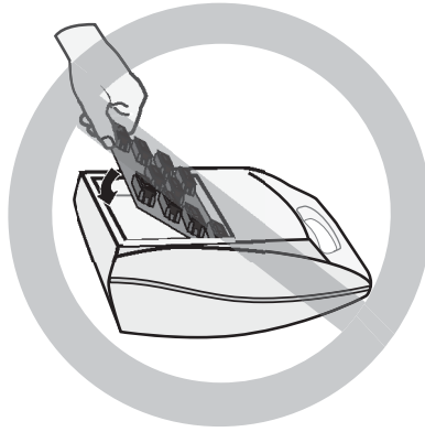
Figure 10: DO NOT install battery assembly this way.
