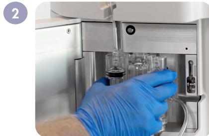
2 Load cartridge, spike IV bag, plug in transducer cable, select "PREP" to ready cartridge for use
