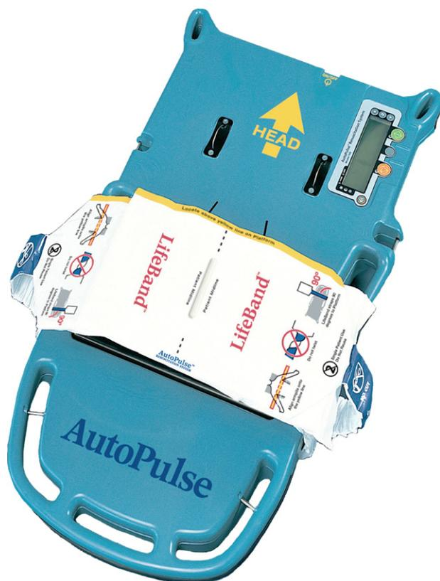
**Figure 1** The AutoPulse™ portable board has a size of ~100 cm × 60 cm and contains a motor to retract the broad load-distributing band (lifeband) under microprocessor control.
