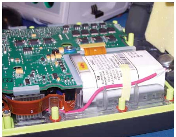
No water damage as the device is opened.
