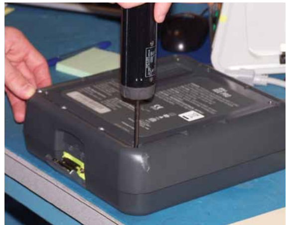
Opening the device for the first time after it was submerged.
