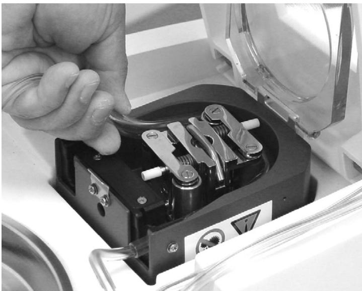
Figure 4.41. Pump Tubing Installation
