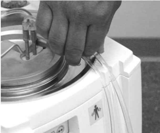
Figure 4.46. Route the Tubing Out of the Console
