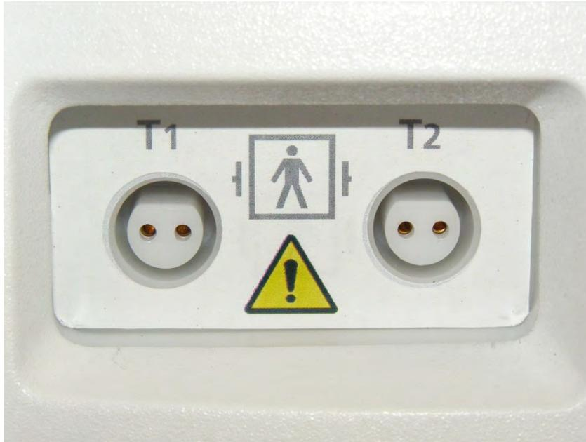
Figure 2.4. Temperature Probe Connectors.
