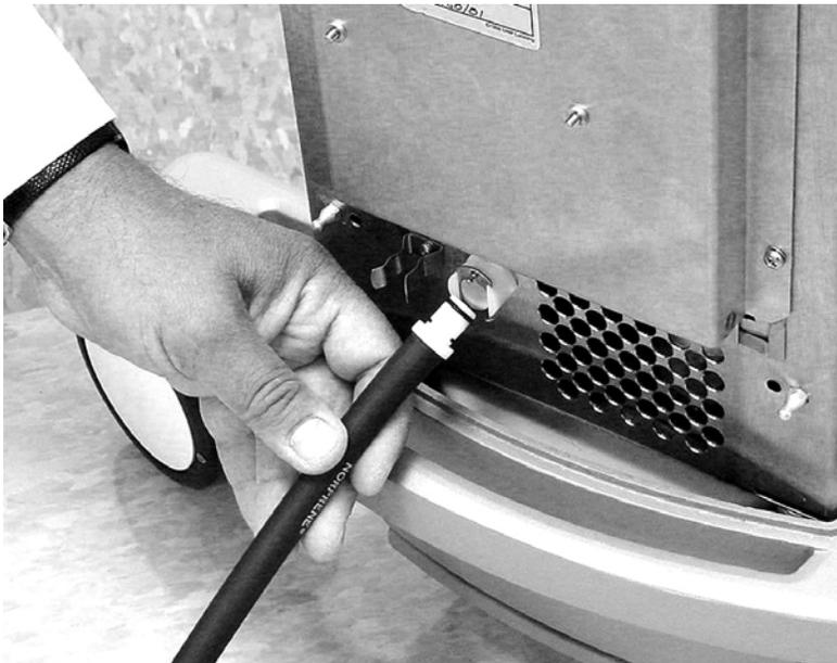
Figure 7.3. Push Hose Into Drain Coupler
