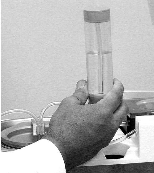
Figure 4.44. Hold the Air Trap Upside Down
