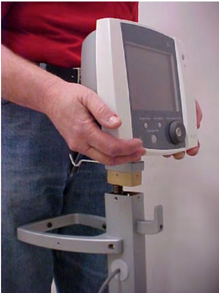
Figure 3.4. Attach the Display Head to the Mast
