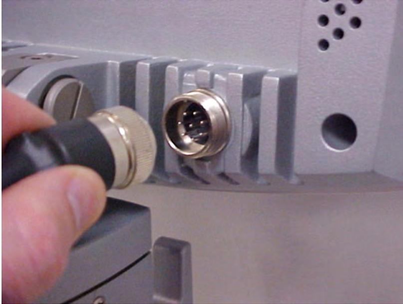
Figure 3.5. Plug the Control Cable Into the Socket
