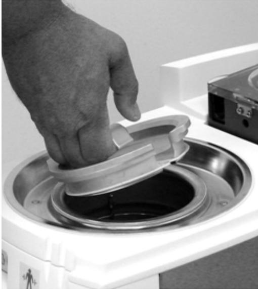
Figure 4.34. Coolant Well Cap
