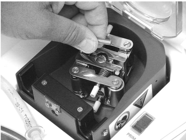
Figure 4.39. Lift the Pump Rollers Handle
