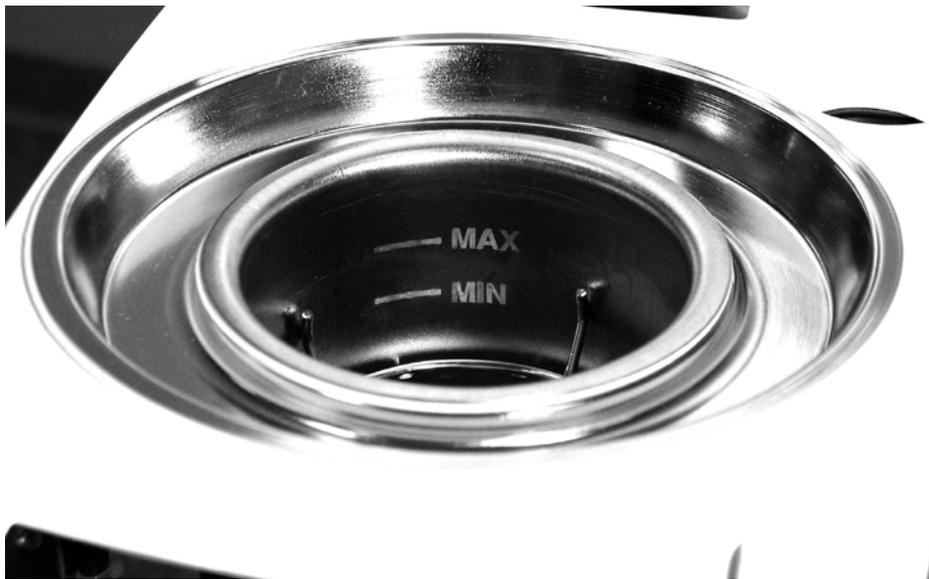
Figure 4.35. Coolant Well Liquid Level Indicator Lines
