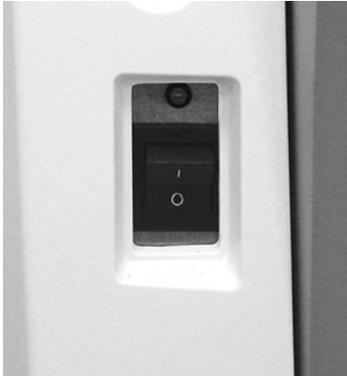
Figure 4.21. Power Switch and Power Indicator Lamp
