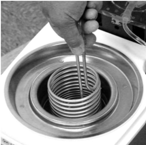
Figure 4.37. Installing the Heat Exchange Coil
