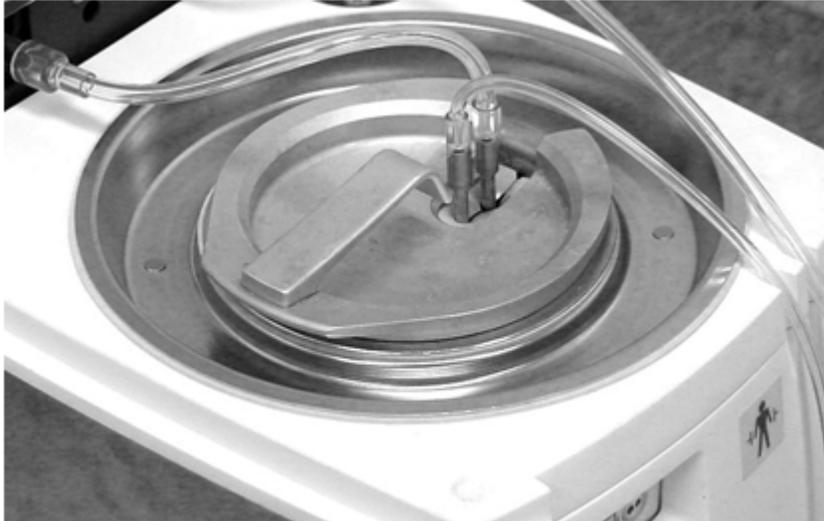
Figure 4.42. Replace the Cap on the Coolant Well
