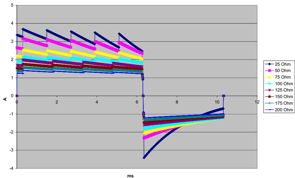
Figure A-18. Rectilinear Biphasic Waveform at 3 Joules
