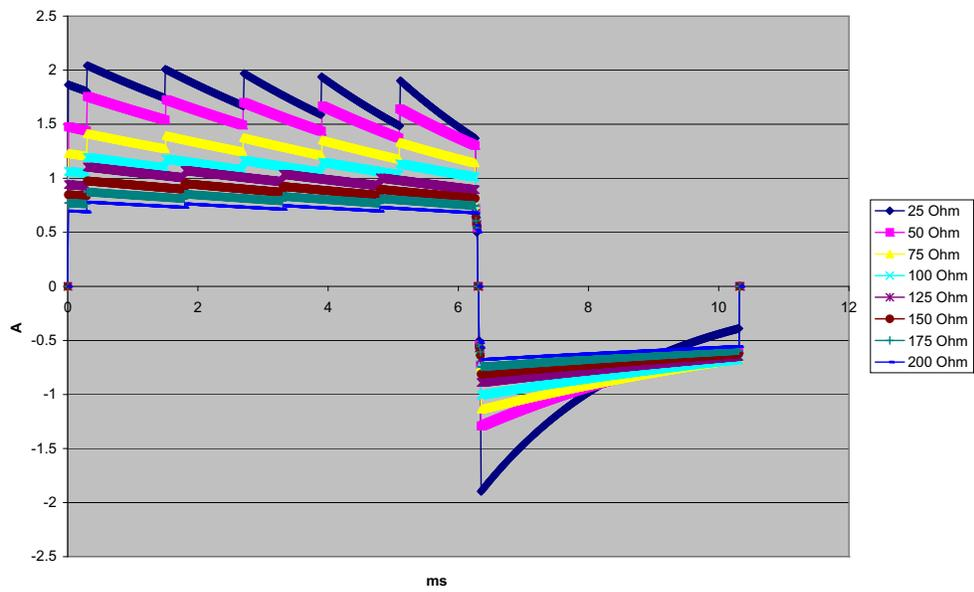
Figure A-20. Rectilinear Biphasic Waveform at 1 Joule
