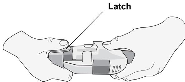
When disconnecting the OneStep electrode and OneStep cable, press down the latch with your thumb as shown.
