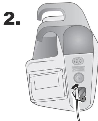
**Figure 9-1 Connecting the Sampling Line Connector to the CO<sub>2</sub> Inlet Port**
