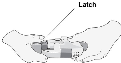
When disconnecting the OneStep electrode and OneStep cable, press down the latch with your thumb as shown.
