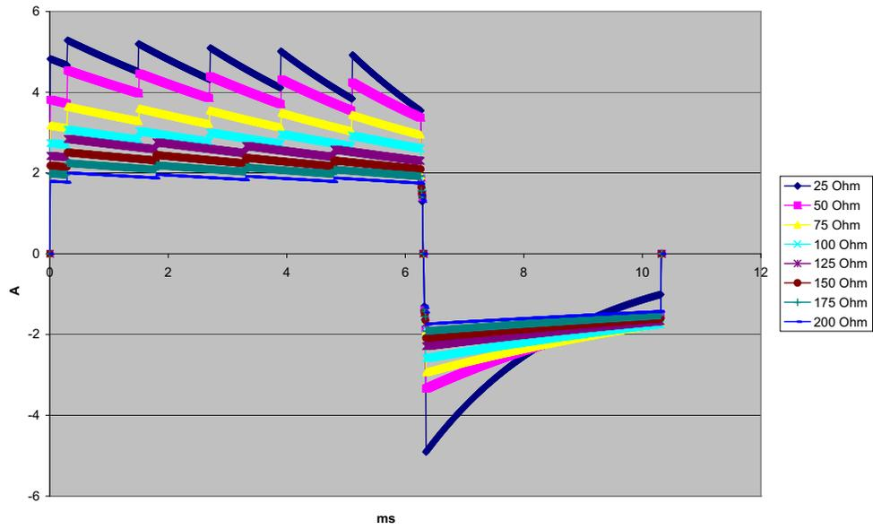
Figure A-15. Rectilinear Biphasic Waveform at 6 Joules
