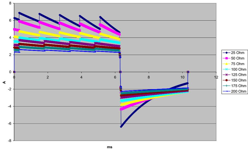
Figure A-11. Rectilinear Biphasic Waveform at 10 Joules
