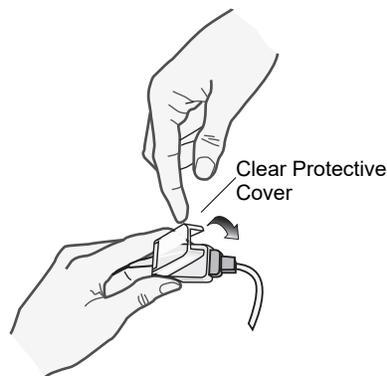
**Figure 10-2 Lower Plastic Cover Over Cable Connection**
