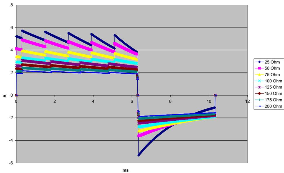
Figure A-14. Rectilinear Biphasic Waveform at 7 Joules
