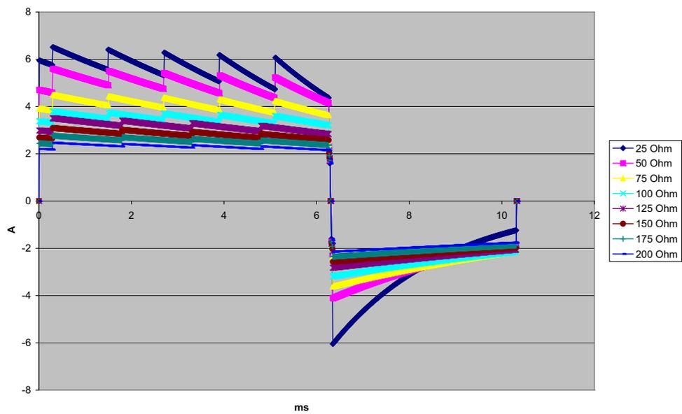
Figure A-12. Rectilinear Biphasic Waveform at 9 Joules
