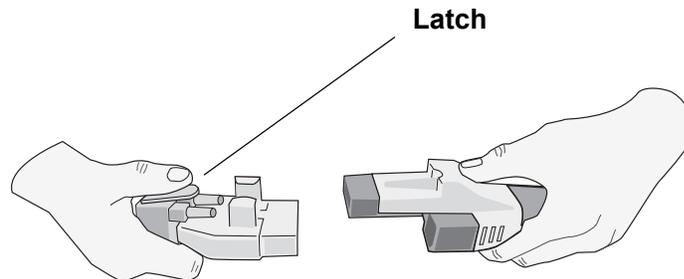
When attaching the OneStep cables to paddles, attach the OneStep cable from the Propaq MD unit to the connector at the base of the apex paddle.
