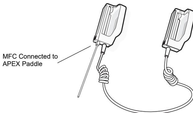
**Figure 2-7. MFC Connected to APEX Paddle**
