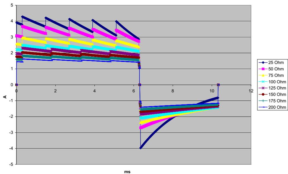
Figure A-17. Rectilinear Biphasic Waveform at 4 Joules
