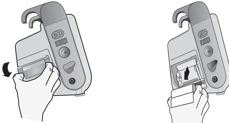
**Figure 24-1. Opening the Printer Door and Removing Paper**
