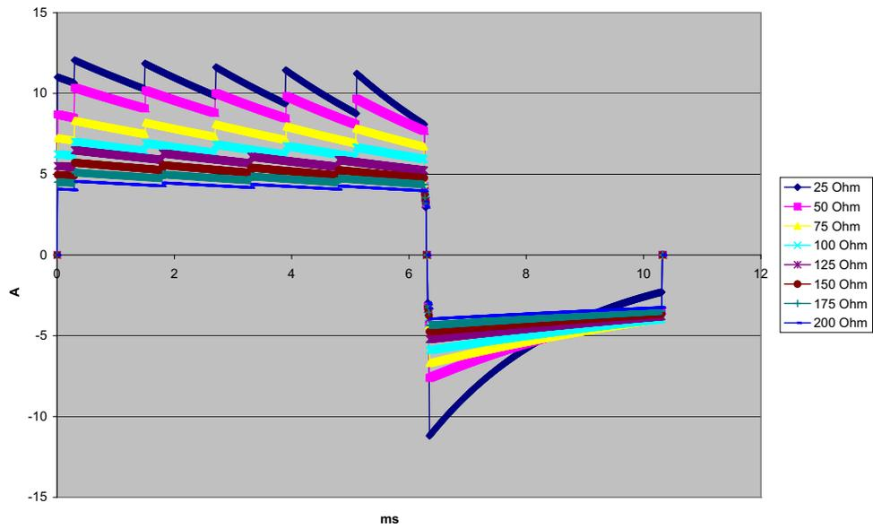
Figure A-8. Rectilinear Biphasic Waveform at 30 Joules
