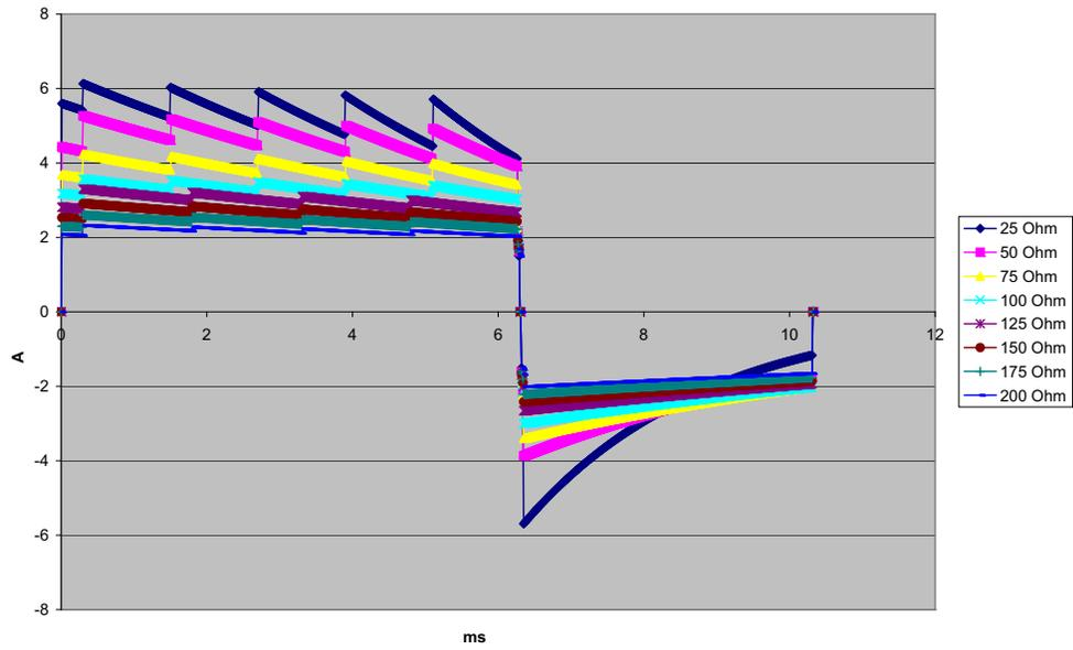
Figure A-13. Rectilinear Biphasic Waveform at 8 Joules
