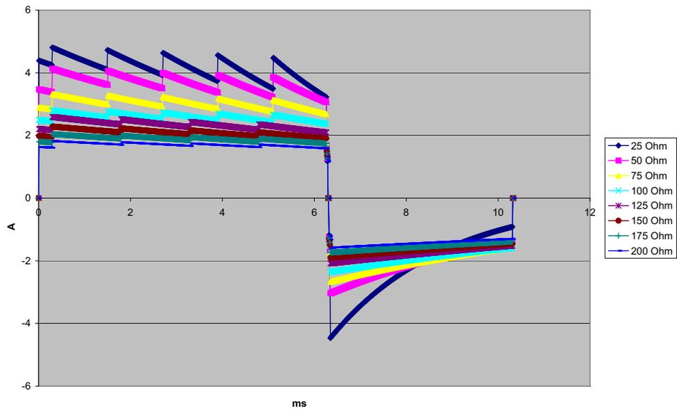
Figure A-16. Rectilinear Biphasic Waveform at 5 Joules
