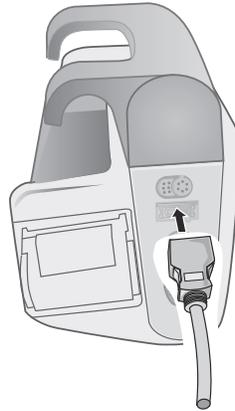
Figure 10-3 Connecting the SpO<sub>2</sub> Sensor to the Propaq MD Unit
