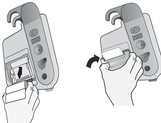
**Figure 24-2. Inserting the Paper and Closing Printer Door**
