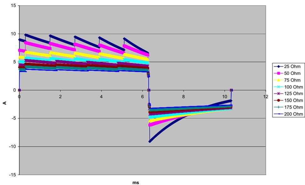
Figure A-9. Rectilinear Biphasic Waveform at 20 Joules
