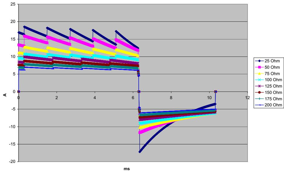
Figure A-6. Rectilinear Biphasic Waveform at 70 Joules
