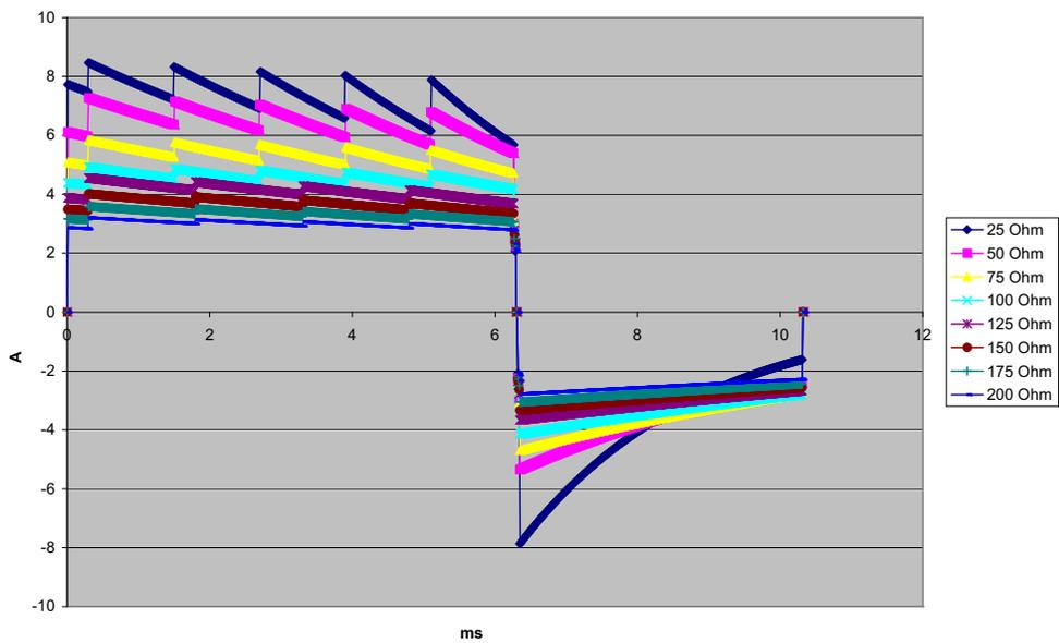
Figure A-10. Rectilinear Biphasic Waveform at 15 Joules
