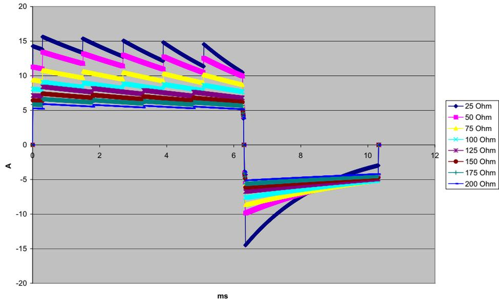
Figure A-7. Rectilinear Biphasic Waveform at 50 Joules
