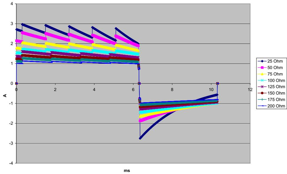
Figure A-19. Rectilinear Biphasic Waveform at 2 Joules
