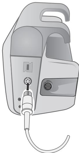
**Figure 11-1 Plugging the Transducer into the Propaq MD**
