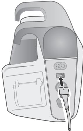
**Figure 9-1 Connecting the SpO<sub>2</sub> Sensor to the Propaq MD Unit**
