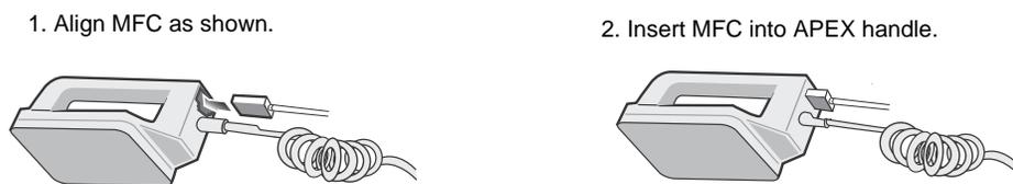
**Figure 2-6. Attaching the MFC to the APEX Paddle**
