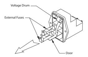
Place the voltage drum back into the Power Module. Close the door. Make sure the voltage setting appears in the window of the door.
