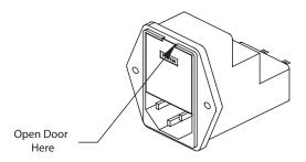
Remove the voltage drum from the Power Module by pulling straight out. Set the voltage drum to the appropriate voltage setting by turning the voltage drum.
