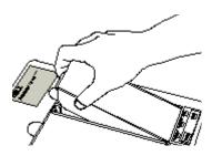
3. Press the **TEST** button. The **TESTING** indicator light will illuminate for the duration of the test cycle.
